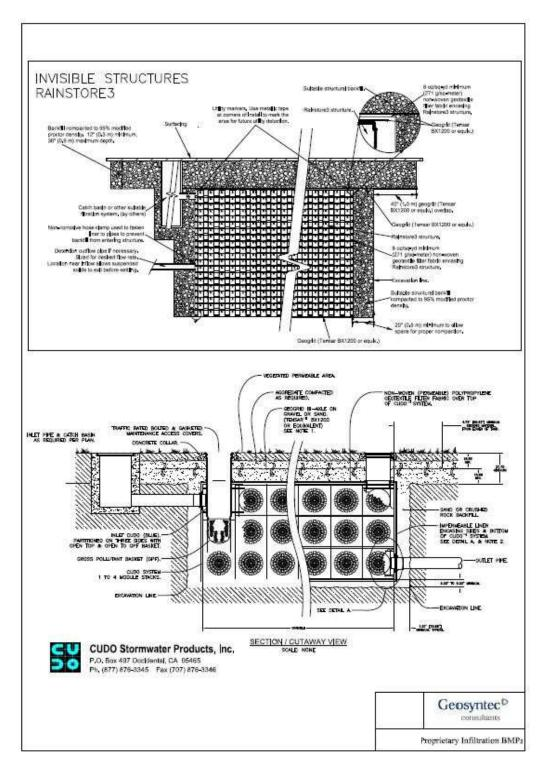
Figure 9. Subsurface Infiltration System (INF-6) Concept
