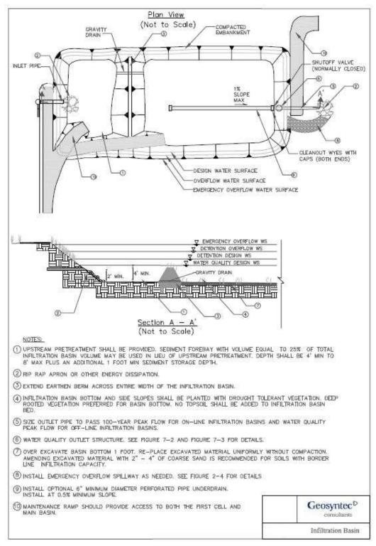
Figure 7. Infiltration Basin (INF-1) Concept
